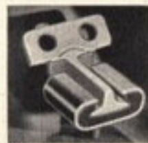
Steel-encased rubber mountings absorb vibration, hold engine steady in frame.
